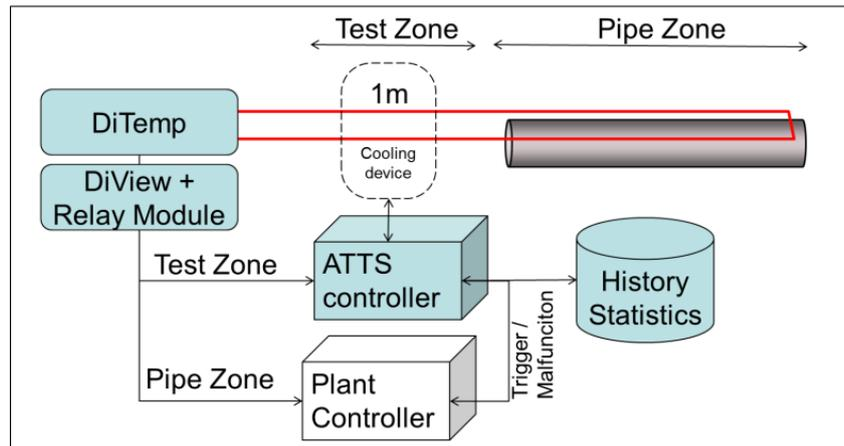
Fig. 5: ATTS block diagram
