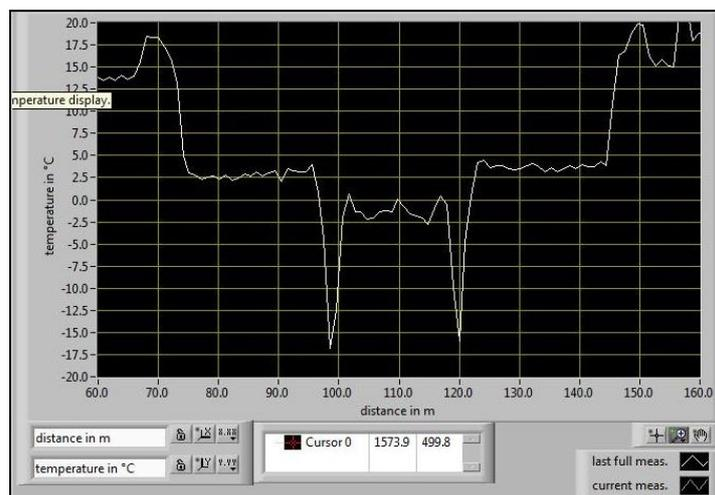
Fig. 7: Plot of temperature as a function of distance during leak test
