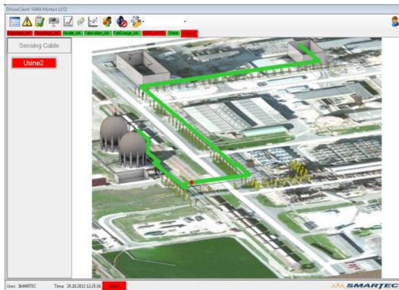
Fig. 3: Example of user interface showing location of event, e.g. leak
