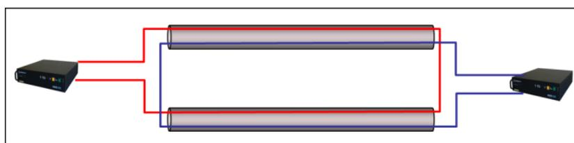
**Fig. 4: Redundant setup with two interrogators and looped fibers**
