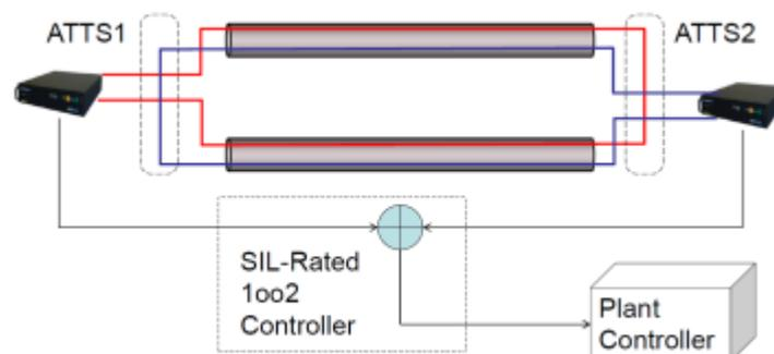
Fig. 8: Redundant system with 2 DTS, 2 ATTS and a voting device
