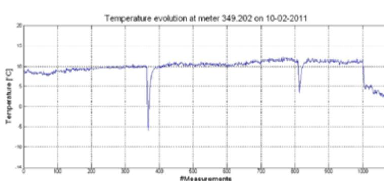
Fig. 6: Temperature drop recorded during two ammonia leak tests and a pipeline restart
