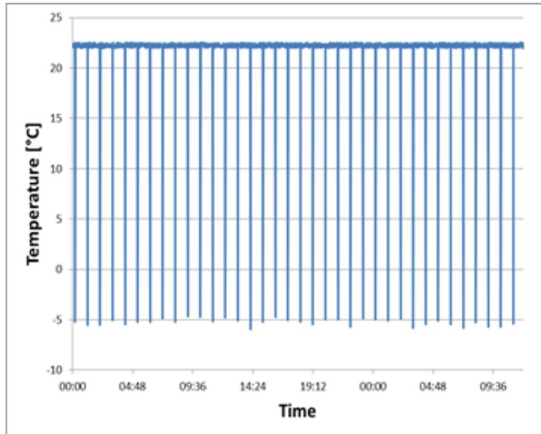
Fig. 7: Example of ATTS temperature recording at the cooling location
