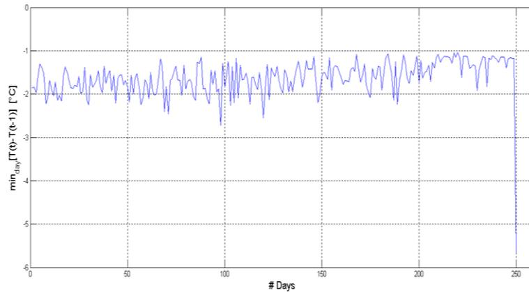
**Fig. 8: Maximum daily rate of change without leaks and with a leak test at the end**
