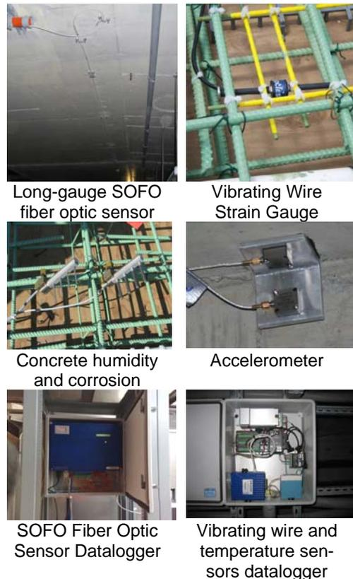
Figure 7: Sensing components
