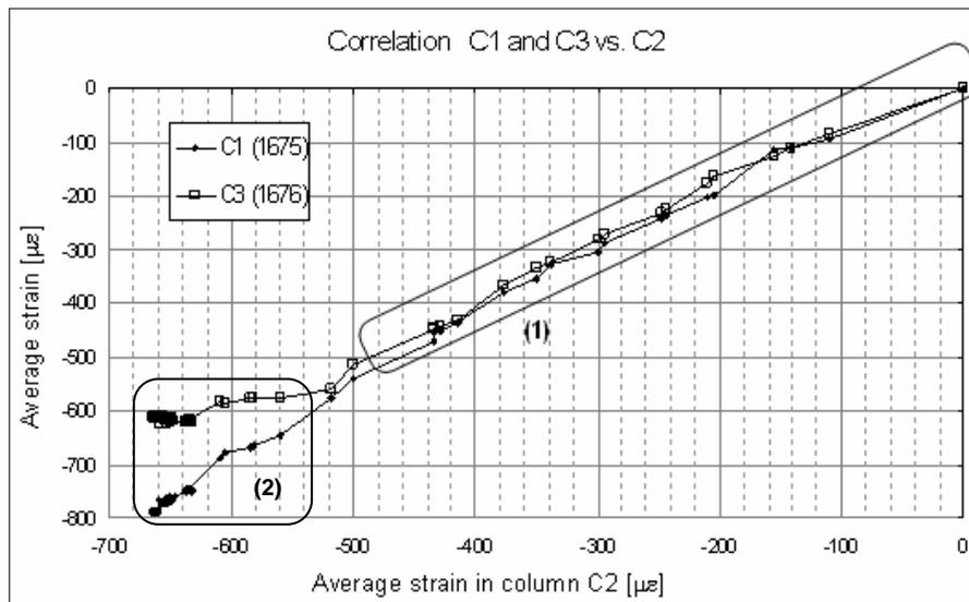
Figure 6. Correlation between column C2 and other columns; highlighted period: (1) construction of 19 storeys; (2) loss of linearity
