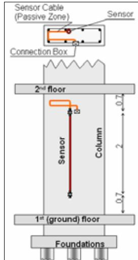
Figure 2. Sensor position in column
