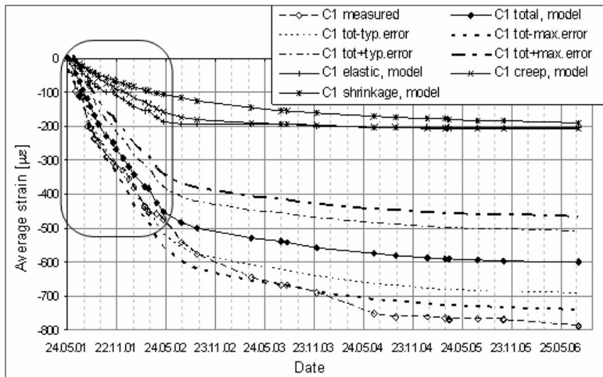
Figure 5. Comparison between the design model and results for column C1
