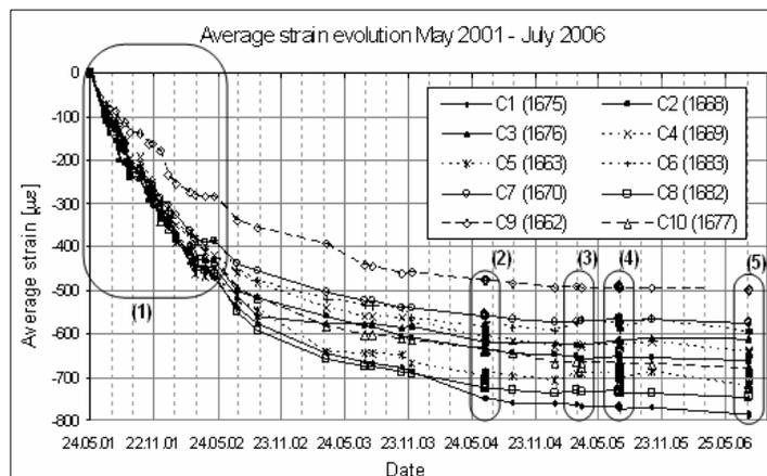
Figure 4. Evolution of total average strain in columns monitored over five years
