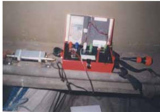
Fig. 16. Peak strain data retriever
