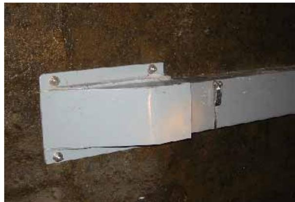
Fig. 28. The tip-end of the sensor protector
