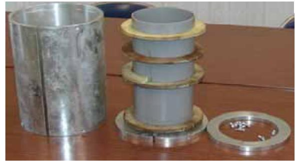
Fig. 13. Sensor bobbin and steel cover
