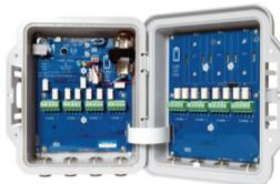
Data can easily be retrieved in **Hz** and **Engineering Units** on your laptop via USB cable. The logger manager software saves all the reading in a text file (CSV), easily imported into your spreadsheet software.
