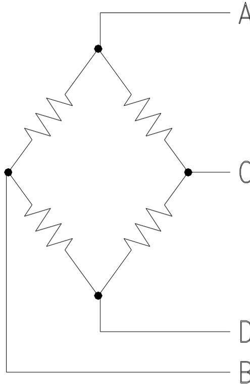
**FIGURE 3: ANCLO Load cell wiring diagram (Full Bridge Configuration).**
