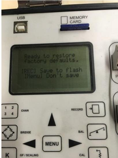
Then press the record button on the front panel to restore factory defaults.
