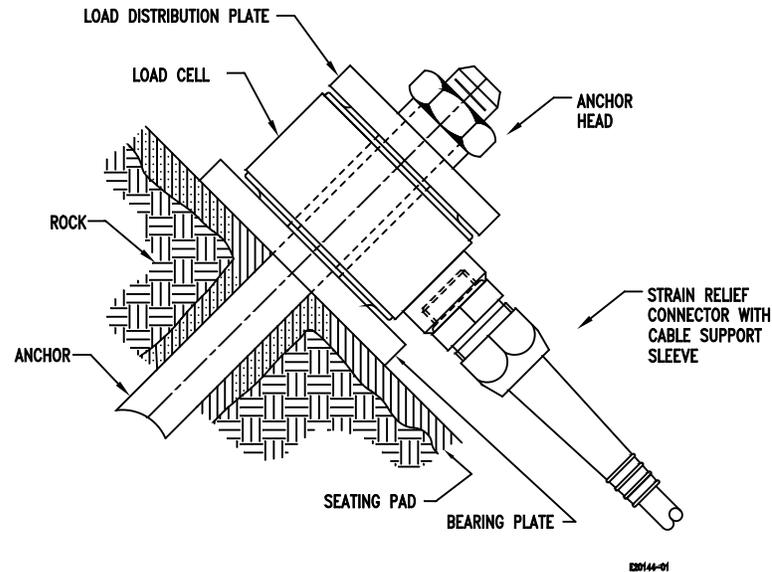
**Figure 1: Anclo typical installation on a tie-back**
