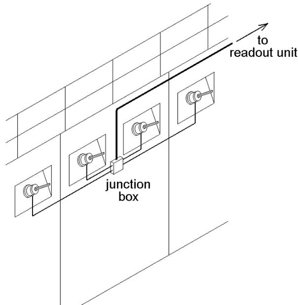
**Figure 2: Example of junction box use**
