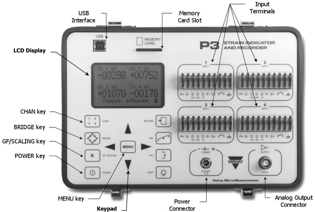
If you want to see the reading of the load cell directly in engineering units as kN then refer to the following instruction for P-3 configuration. You can connect up to four load cells to a P-3 readout unit as it has four channels available.
