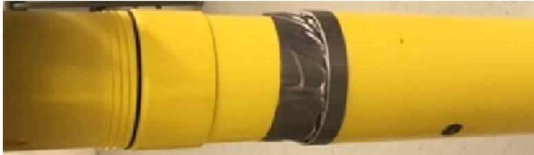
Two layers of duct tape will increase resistance to compression by about 20 kg.
