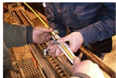
MuST FBG Long Base Sensor 1 m
