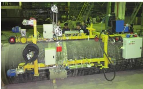
Figure 6: Automated sensor installation machine (courtesy of Laser Solutions, Russia)
