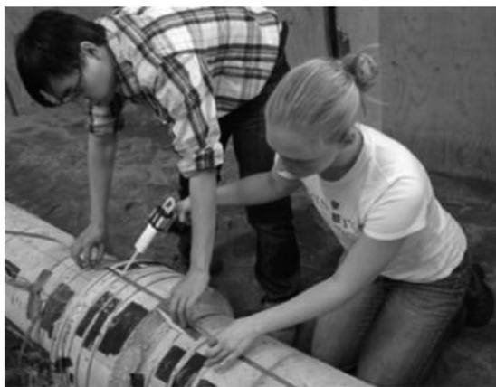
Figure 14: Installation of sensor across a pipe joint. Courtesy of Prof. Branko Glisic (Glisic & Yao 2012)
