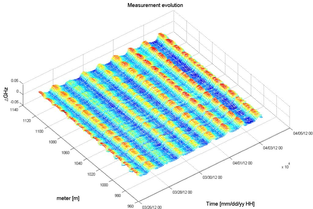
Figure 7. Recorded deformations on a levee wall as a function of position and time.
