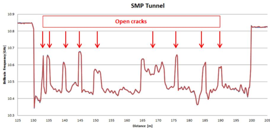
Figure 12 SMARTprofile strain distributed measured along the penstock access tunnel.
