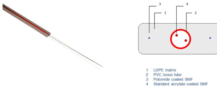
Figure 2. SMARTprofile - combined Strain and Temperature sensor.
