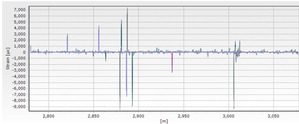
Figure 5. Strain variations in a localized section of the San Salvatore Tunnel. Strain peaks are correlated with small crack movements.
