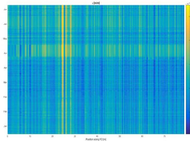
Figure 8. Pseudo color plot of strain versus time (vertical) and position (horizontal).
