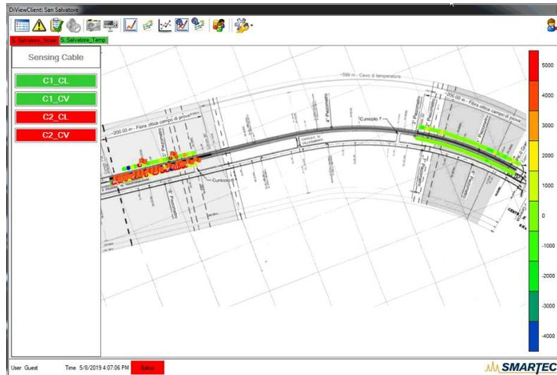
Figure 2. Examples User Interface for distributed monitoring of a tunnel (San Salvatore Tunnel, see below for details), colors indicate level of strain recorded as a function of position. Two sections are instrumented in this case.
