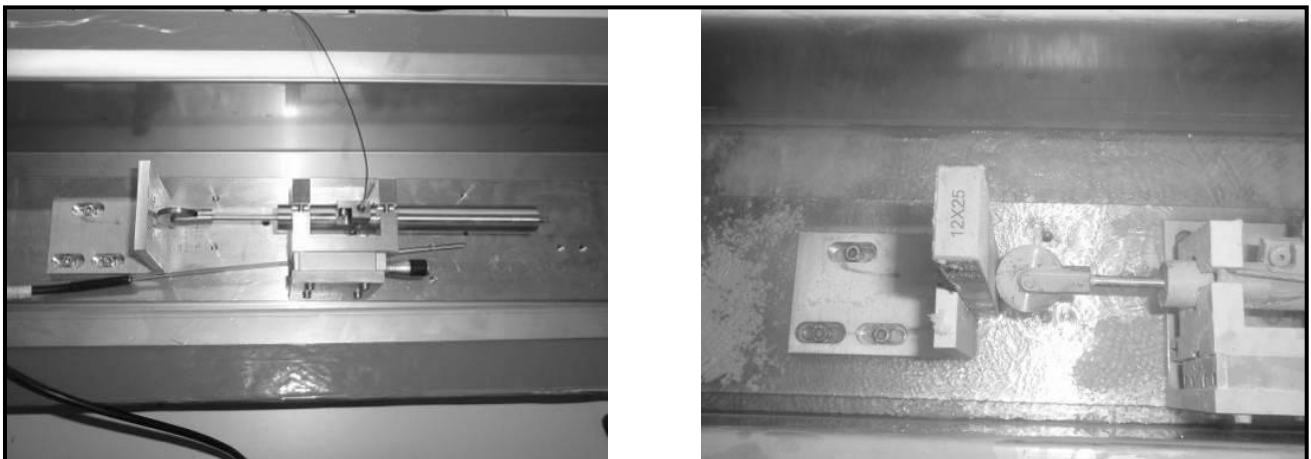
Figure 9. Fibre Optic sensors during the testing campaign.
