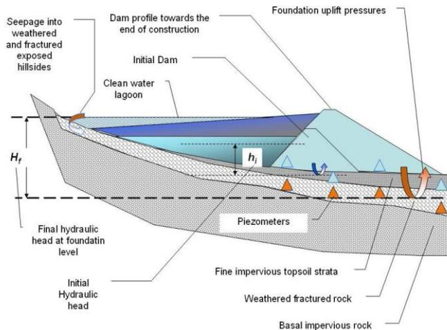
*Figure 11: the hydraulic conditions of a tailing dam*
