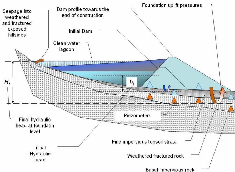
Figure 6. The hydraulic condition of a tailing dam.
