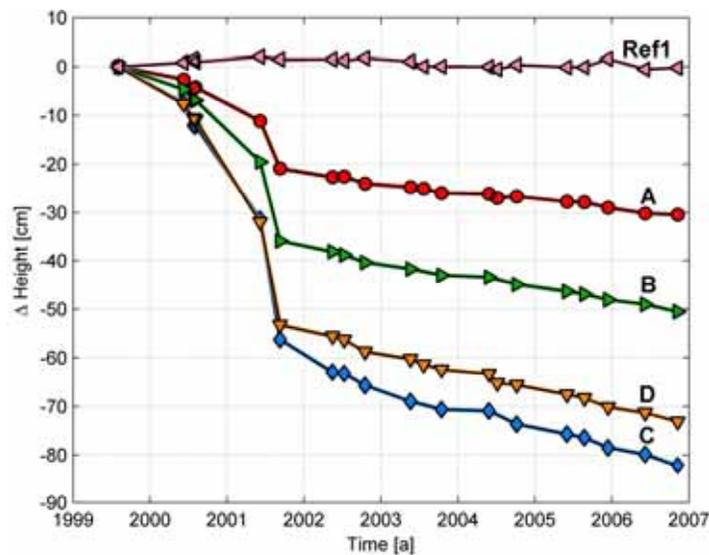
Figure 2. Time series of GPS results for station heights
