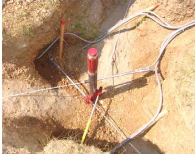
Figure 5. Central tube of the strain rosette during installation
