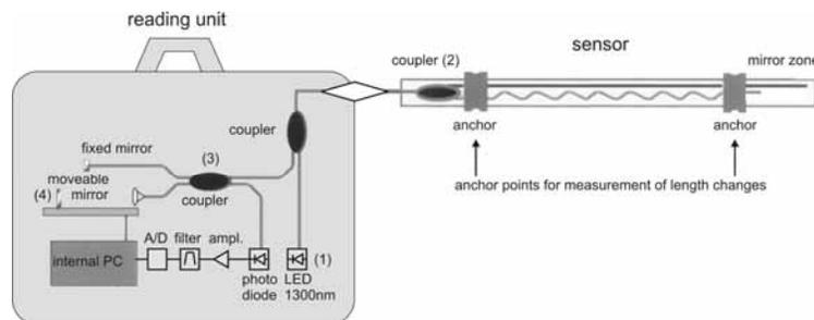
Figure 3. Components of the SOFO-Static system, after [8]
