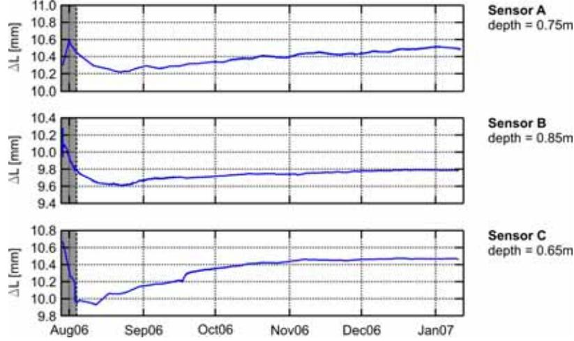
Figure 6. Relative movements of the tubes, determined by the three sensors A, B and C of the strain rosette
