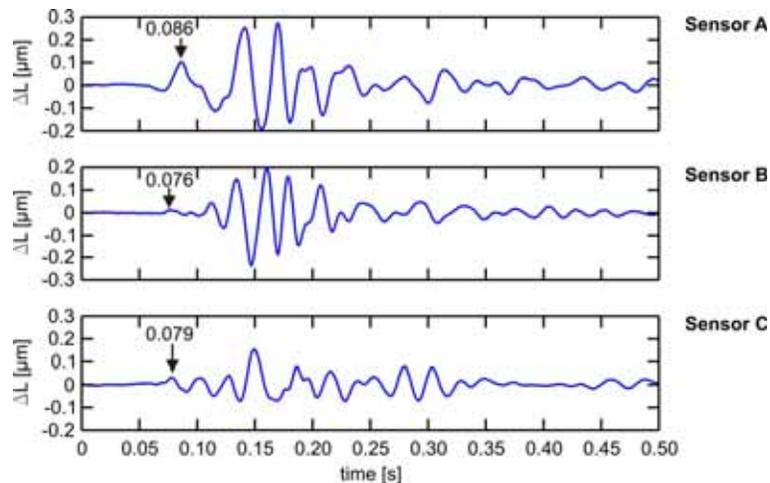
Figure 9. Relative movements of the tubes caused by a hammer impact
