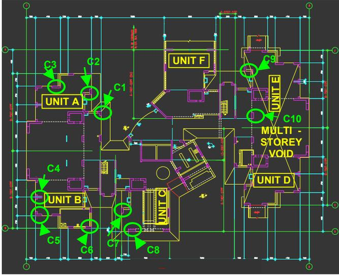
Figure 5. Position of the columns in ground floor equipped with sensors
