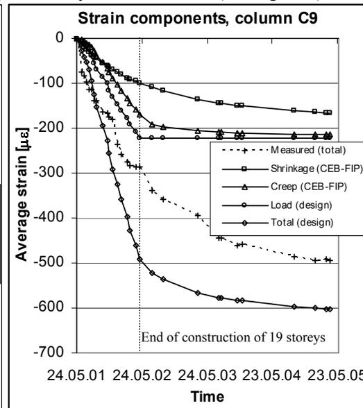
Figure 8. Strain components in column C9
