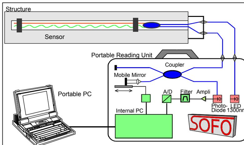
Figure 2. Schema of functioning and components of the SOFO system
