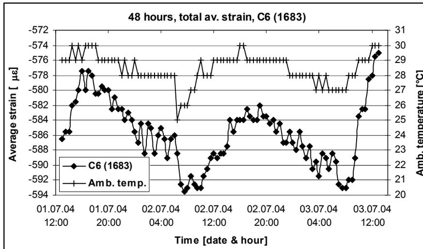
Figure 9. Total average strain and ambient temperature recorded during 48-hours continuous monitoring session performed in July 2004
