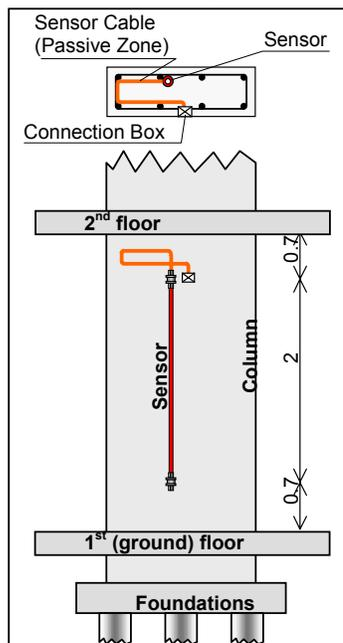
Figure 3. Sensor position in column
