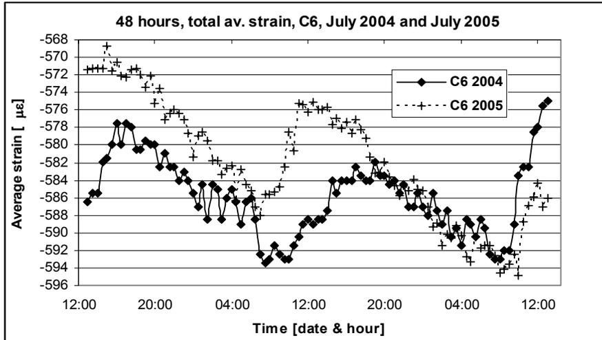
Figure 10. Total average strain in column C6 recorded during 48-hours continuous monitoring sessions performed in July 2004 and July 2005
