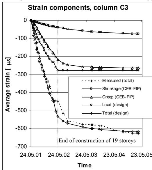
Figure 7. Strain components in column C3
