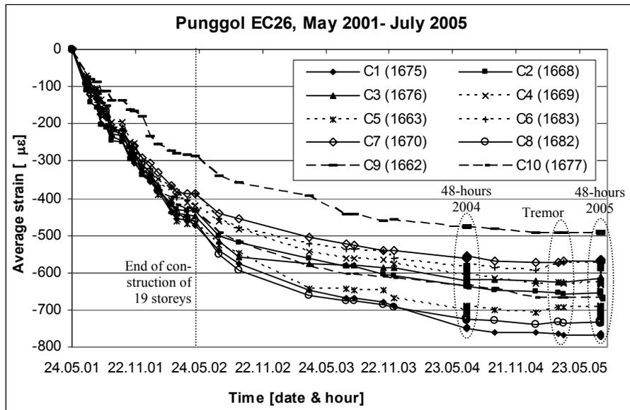
Figure 6. Evolution of total average strain in columns monitored by SOFO system
