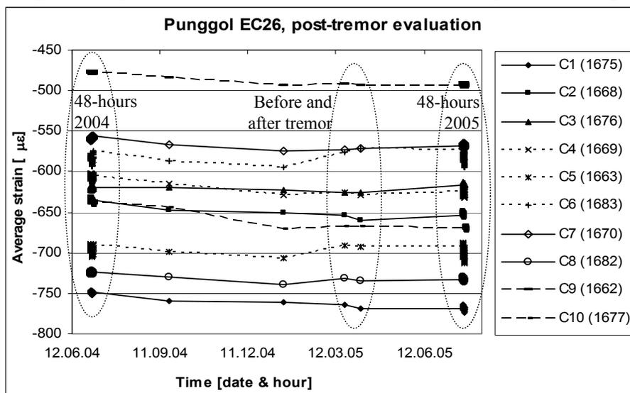
Figure 11: Average strain measurements recorded before and after tremor
