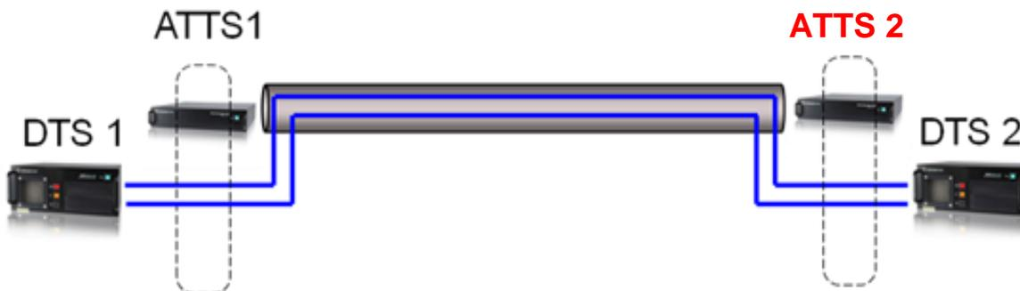
Fig. 5: Example of fully redundant leak detection system with self-testing capability
