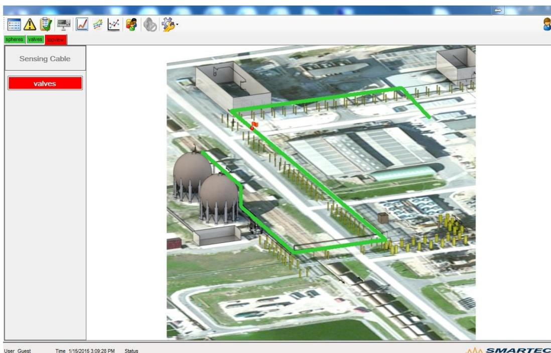
Fig. 2: Example of user interface showing location of event, e.g. leak detection
