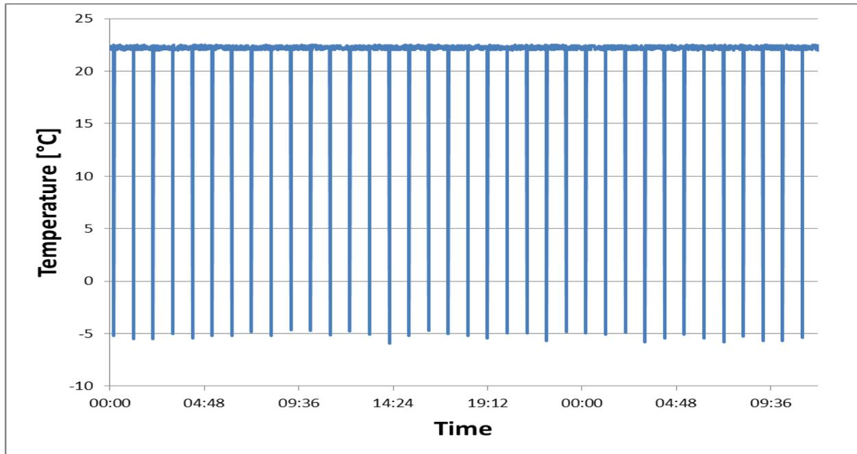
Fig. 9: Example of ATTS temperature recording at the cooling location
