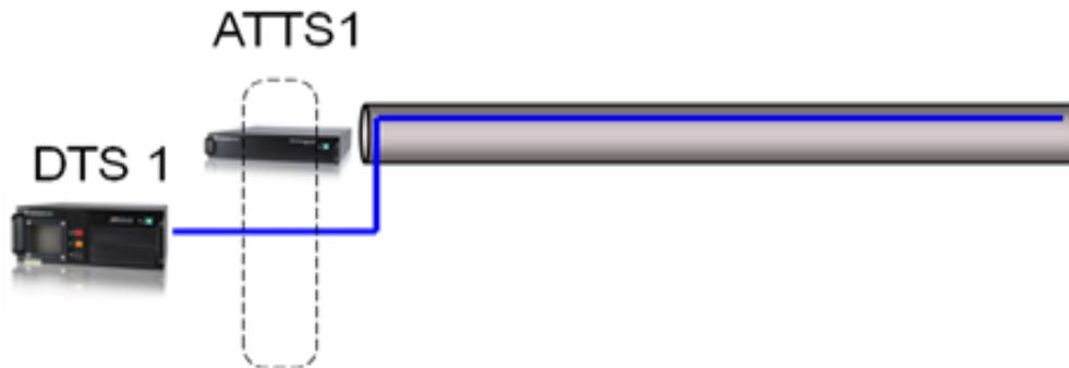
Fig. 4: Example of simple leak detection system with additional self-testing capability
