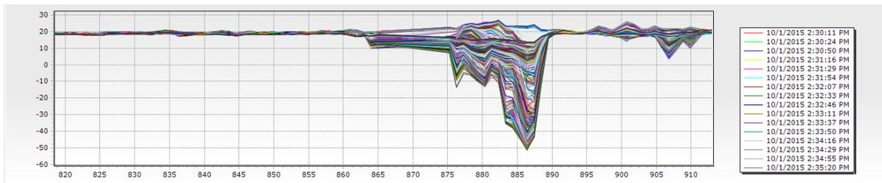
Fig. 7: Temperature distribution along the sensing cable during a leak
