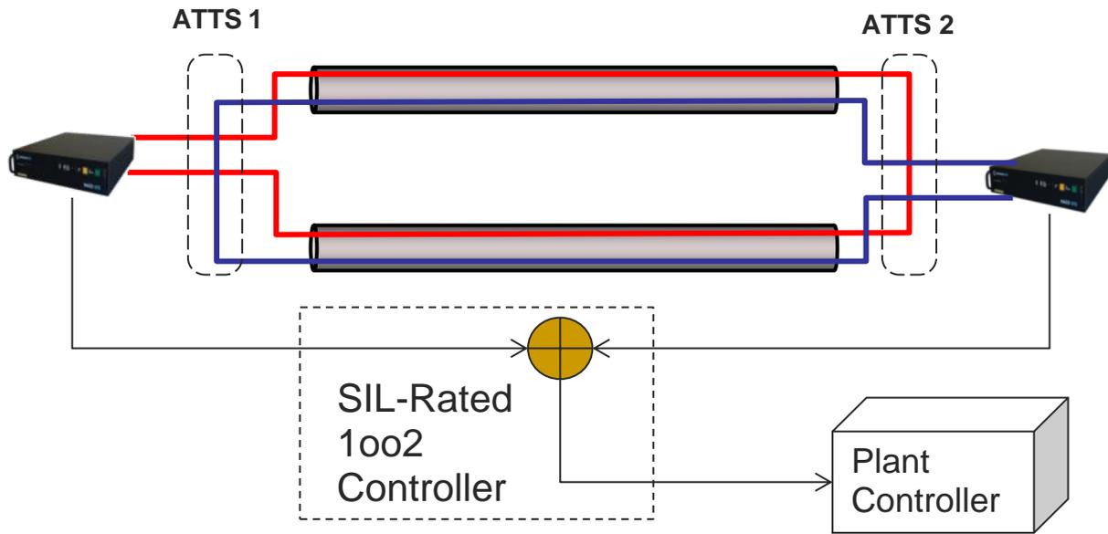
Fig. 6: Example of fully redundant leak detection system with voting system
