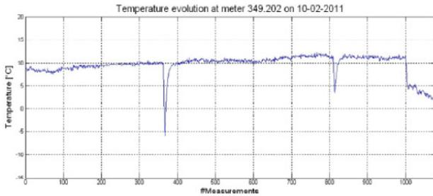
Figure 6. Temperature drop recorded during two ammonia leak tests and a pipeline restart
