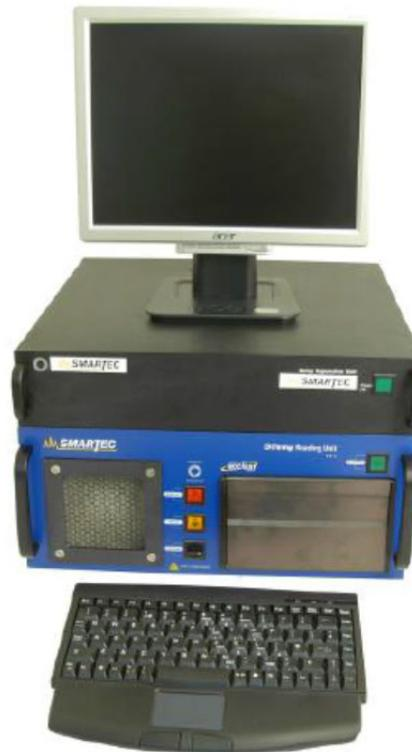
*Figure 1. Distributed temperature sensing interrogator*
