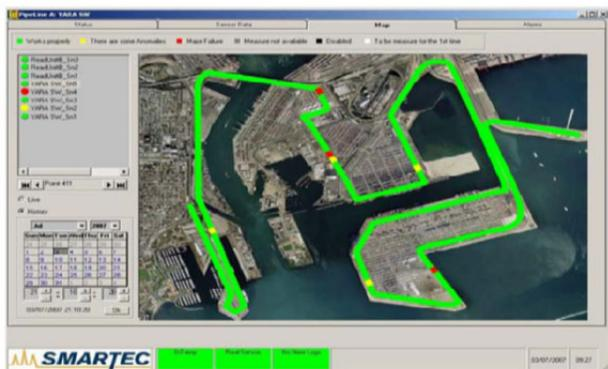
Figure 3. Example of user interface showing location of multiple events, e.g. leaks
