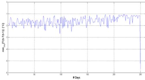
Figure 8. Maximum daily rate of change without leaks and with a leak test at the end
