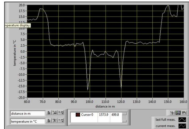
Figure 7. Plot of temperature as a function of distance during leak test
