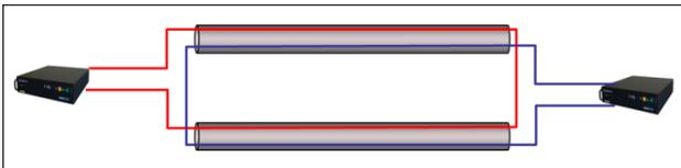
Figure 4. Redundant setup with two interrogators and looped fibers
