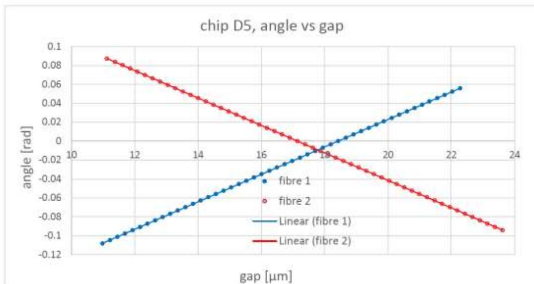
Figure 6. Optical characterization curve for chip D5. Sensitivities are estimated to be  $11.68 \mu\text{rad} / \text{nm}$ .
