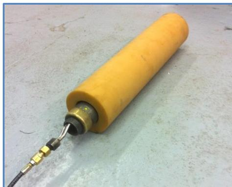
Figure 1. Pressuremeter Probe in the Polyurethane Tube
