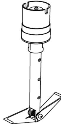
PLUG GROUT VALVE WITH QUICK CONNECT
