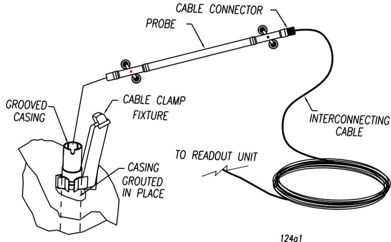
**FIGURE 2: Inclinometer probe insertion into GEO-LOK casing**
