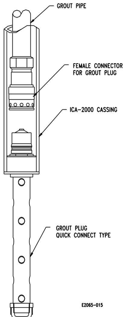
**FIGURE 8: Grout plug assembly**
