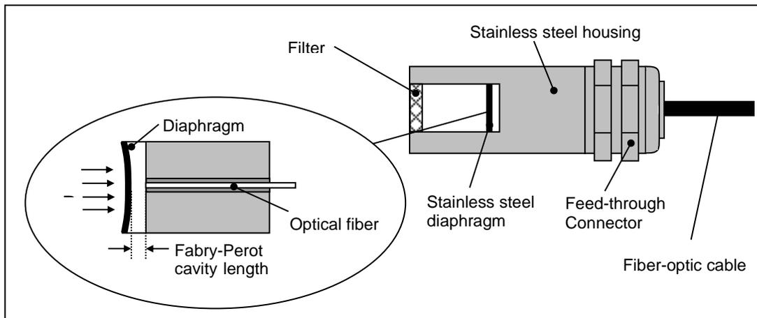
The mechanical robustness of the sensor is assured by the all welded stainless steel construction, with no epoxy, sealing rubber, or other sort of polymeric materials.
