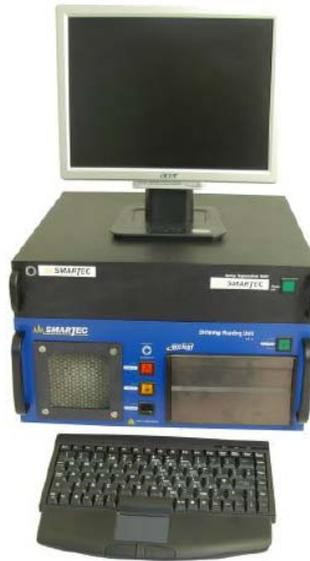
Figure 1. Distributed temperature sensing interrogator
